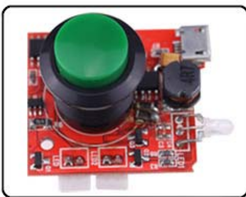
Constant current and voltage controll, can procect LED and battery
